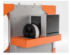
The spool holder has been designed to fit all standard spool sizes. It can hold two spools of up to 8 kg. An in-built detection system notifies the user when the filament is about to end. Optionally a filament enclosure box is available to protect filament from dust and moisture.
