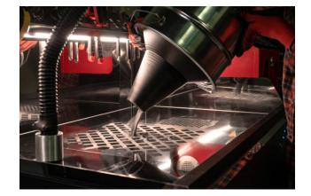
All the recovered powder is transferred to a sieving module and then goes into a metal container. Now it's ready to reuse
