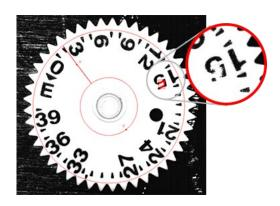
Flexible Flaw Detection is ideal for edge- and area-based inspection of shapes. To find edges and boundaries under error-prone conditions, FFD compares edges in a trained model to edges in the run-time image to check for extra or missing edges. FFD works for both color and greyscale applications, giving users the flexibility to balance accuracy versus speed, and even to ignore defects during run-time.
