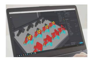
BLADE, BigRep's easy to use slicer software, allows for greater control of printing parameters on all BigRep large-format 3D printers. Its integrated estimation engine gives accurate printing time and material use predictions for unmatched planning and productivity.
