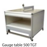
Plate thickness measuring table. Long arm to allow any plate size. Gauge finger by gravity (no pressure). Command by means of foot switch. Possibility of tolerance pre setting with alarm when measure out of tolerance. 100 kgs 121 x 121 x 110 cm 48 x 48 x 43 inch
