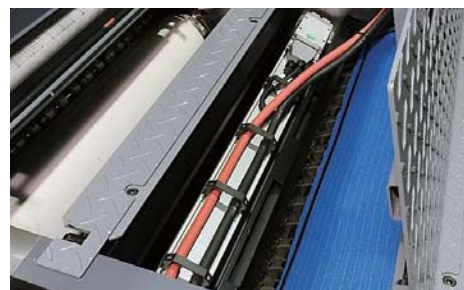
Inter-deck LED-UV curing unit over the impression cylinder
