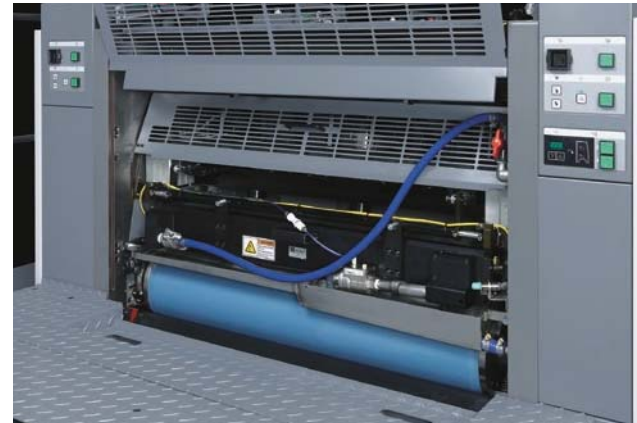
Chamber type coating unit
