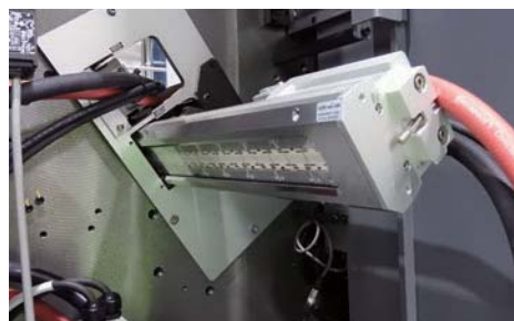
LED-UV curing unit in the delivery section
