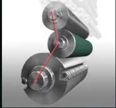
Seven o'clock cylinder arrangement
