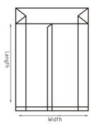
600Z Center Seal: Width 120~600mm Quad Seal: Width 200~360mm Gusset depth: 20~80mm Bag Length: 60~300mm (Up to 6 Skips)
