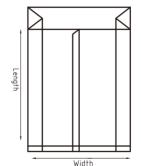
450Z Center Seal: Width 80~450mm Quad Seal: Width 100~200mm Gusset depth: 20~60mm Bag Length: 60~250mm (Up to 6 Skips)
