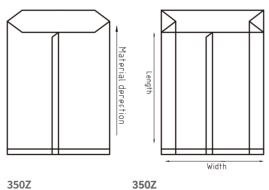
中封袋:袋宽80~350mm 四边封:袋宽100~180mm 风琴插深:20~60mm 风琴抽深:20~60mm Bag Length: 袋长:60~250mm(可做6倍送) 60~250mm (Up to 6 Skips)
