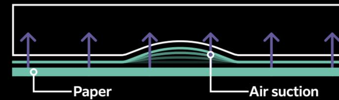
The shuttle head draws up the paper strongly using a small amount of air, separating and delivering each sheet reliably. The active head avoids friction on the paper surface, which can be a problem with other suction feeding technologies.
